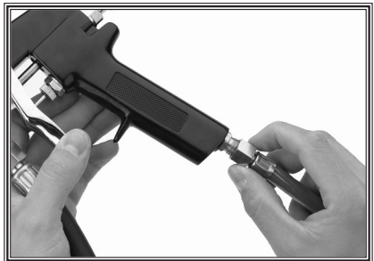
Figure 6. Attaching hose to spray gun.
